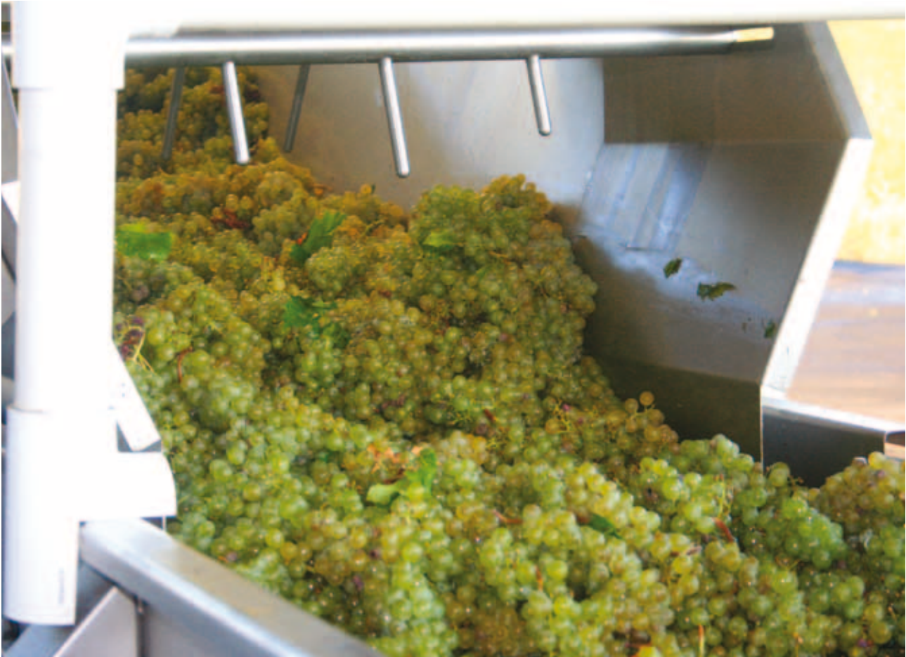
A small amount of SO 2 is added at the crusher, to prevent both enzymatic and chemical oxidation of phenols.
